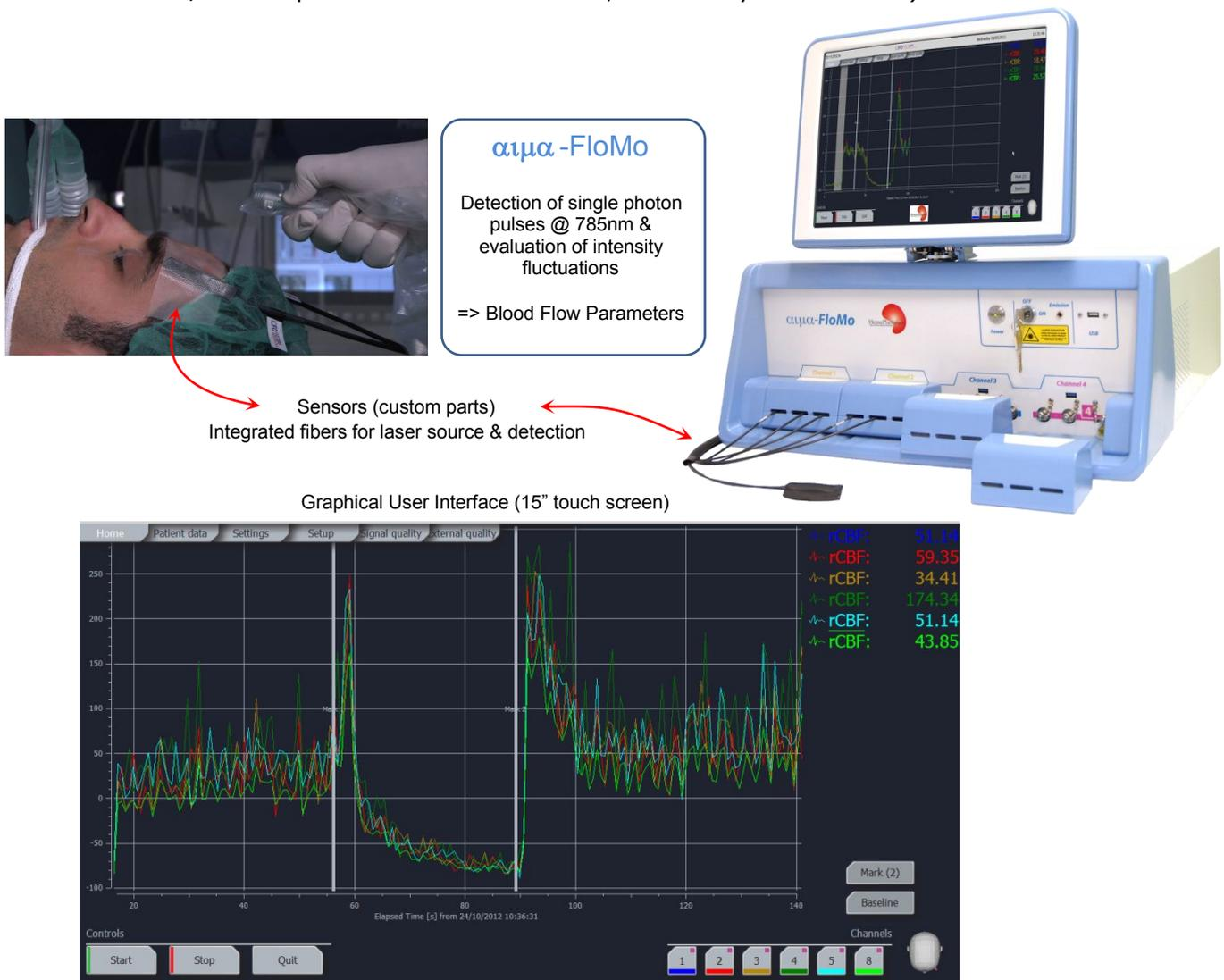
The **αιμα-FloMo** is meant to be used with an NIRS/DOS system and can readily be integrated with most commercial and custom systems. Together with NIRS/DOS, the blood oxygenation and blood volume (Hb, Hb, THb and StO<sub>2</sub>) can be measured as well as the blood flow which allows the derivation of other relative parameters such as the oxygen extraction fraction (OEF) and cerebral metabolic rate of oxygen extraction (CMRO<sub>2</sub>).
